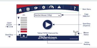
**HMI** – FlexFlow's large, color, touchscreen is as intuitive and user friendly as any smartphone. This easy-to-use and read interface gives access to maintenance operations, animated help screens, and more. It makes working with FlexFlow a breeze.
