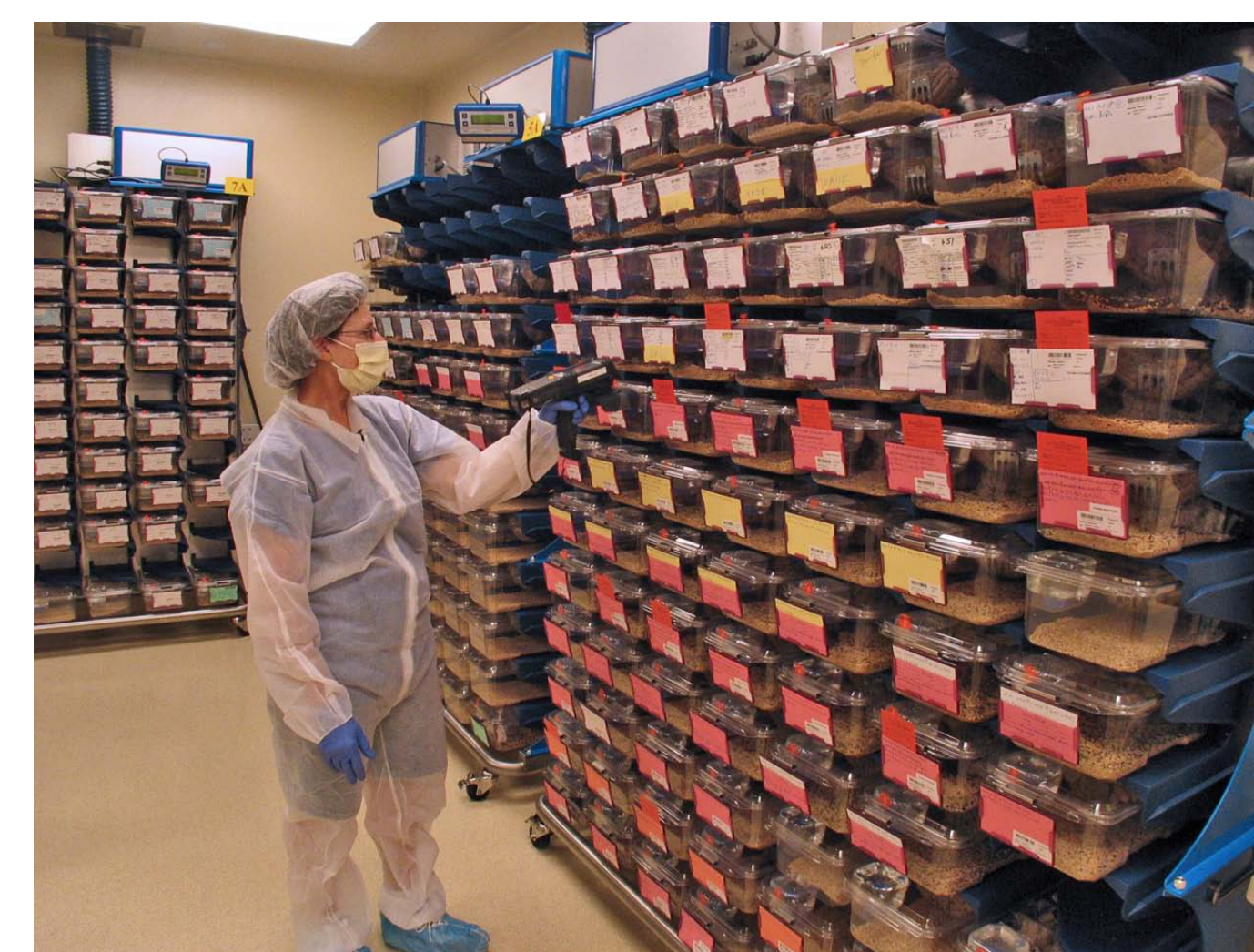
Figure 2. Scanning of RFID tags is done with a handheld device. All cages are associated with a barcoded cage card and RFID card holder.
