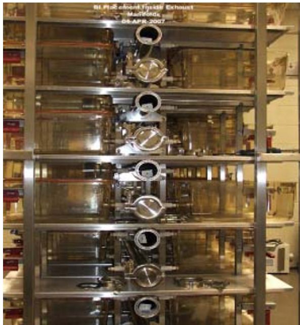
Photo #2: Showing placement of BI's in each exhaust manifold (EX-1 thru EX-7).
