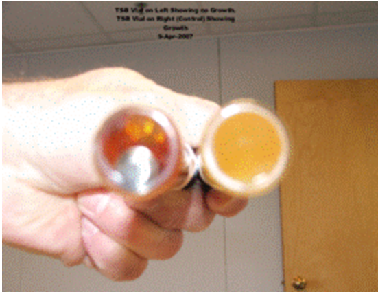
Photo #4: Showing TSB vial on left with no signs of growth. TSB control vial on right showing growth.
