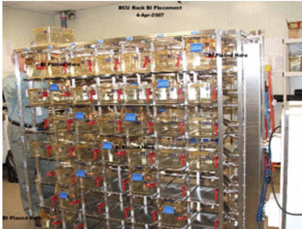
Photo #1: Showing placement of BI's in each corner and middle cages of rack. Same BI placement on both sides of rack. (A1 to G7) & (H1 to N7).
