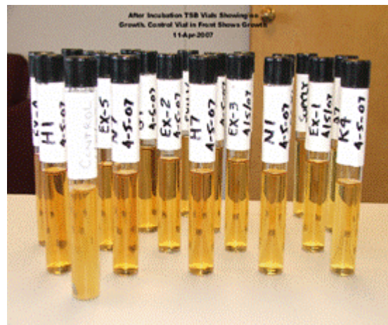
Photo #3: (Lt. 20 TSB vials before incubation Rt. 20 TSB vials after incubation control vial showing growth)
