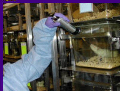
Ammonia Level Testing
